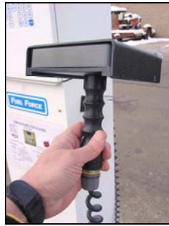
Proximity Reader wand is used to read vehicle tags
