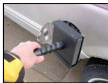
Proximity Reader wand is used to read vehicle tags
